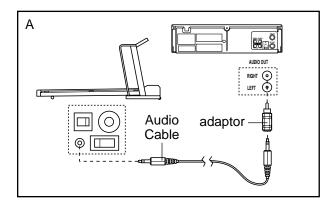
B. Plug one end of the audio cable into the jack on the front of the treadmill near the power cord. Plug the other end of the cable into the included adaptor. Plug the adaptor into an RCA Y-adaptor (available at electronics stores). Next, remove the wire that is currently plugged into the AUDIO OUT jack on your VCR and plug the wire into the unused side of the RCA Y-adaptor. Plug the RCA Y-adaptor into the AUDIO OUT jack on your VCR.
